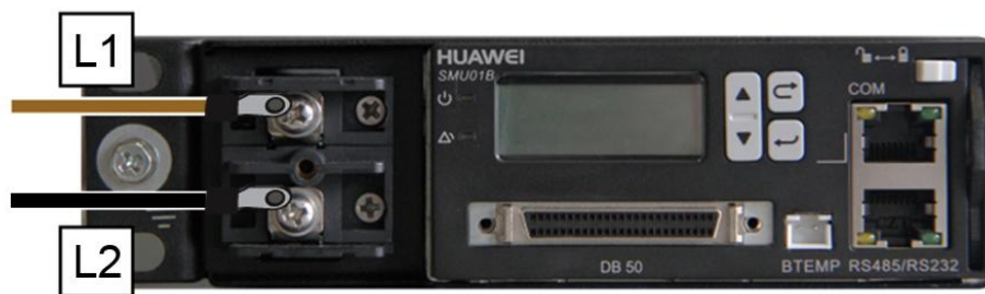
Figure 4-12 Connecting the dual-live wire AC input power cable
