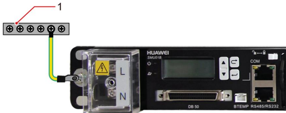
Figure 4-5 Connecting the ground cable
