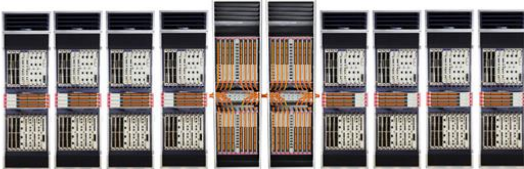
Figure 6 Physical architecture of a CCC-2 system (400G cluster)
