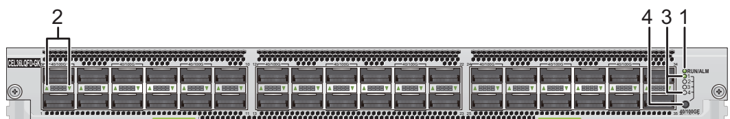
Figure 4-69 Indicators and button on the CEL36LQFD-GK
